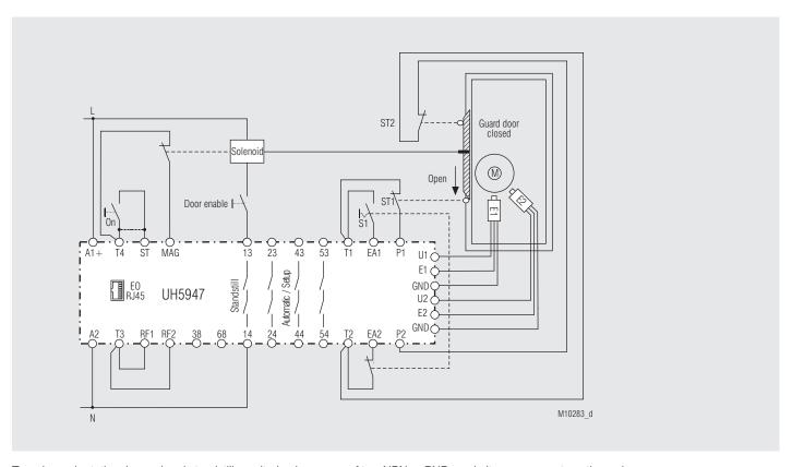
Two-channel rotational speed and standstill monitoring by means of two NPN or PNP proximity sensors; automatic mode; safety gate monitoring active; for manual start: ON/OFF pushbutton to T4/ST; for automatic start: jumper to T4/ST; suited up to SIL 3, Performance Level e (Requirement for Cat4 is, that during longer periods of standstill a forced dynamisation (t<24h) has to be carried out).
