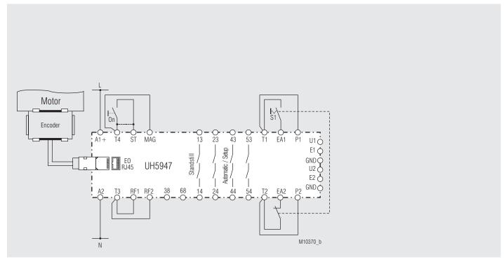
Rotational speed and standstill monitoring with suitable encoder, automatic mode; for manual start: ON/OFF pushbutton to T4/ST; for automatic start: jumper to T4/ST; suited up to SIL 3, Performance Level e (Requirement for Cat4 is, that during longer periods of standstill a forced dynamisation (t<24h) has to be carried out).
